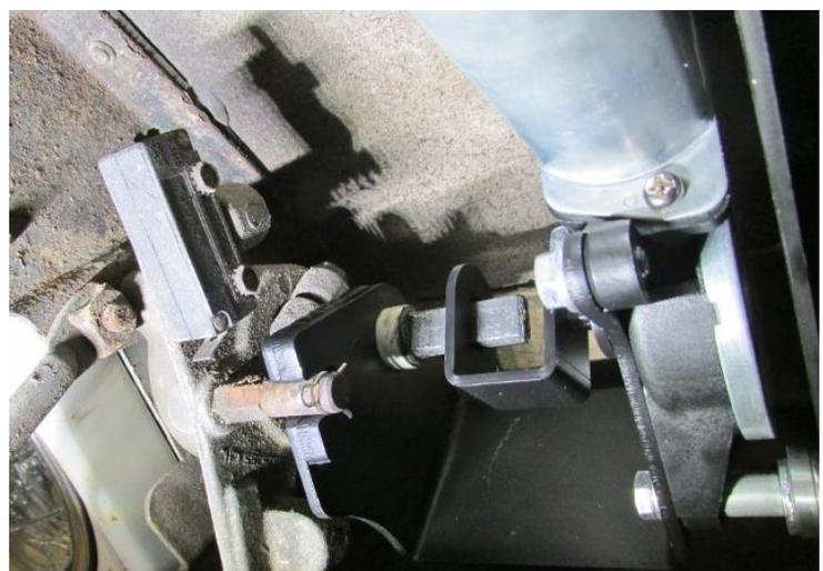
Figure 5 – Install Motor Assembly
