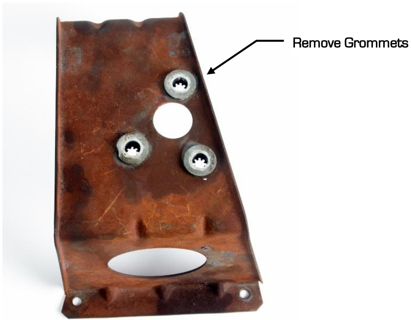
Figure 2 - Factory Wiper Motor Mounting Bracket
