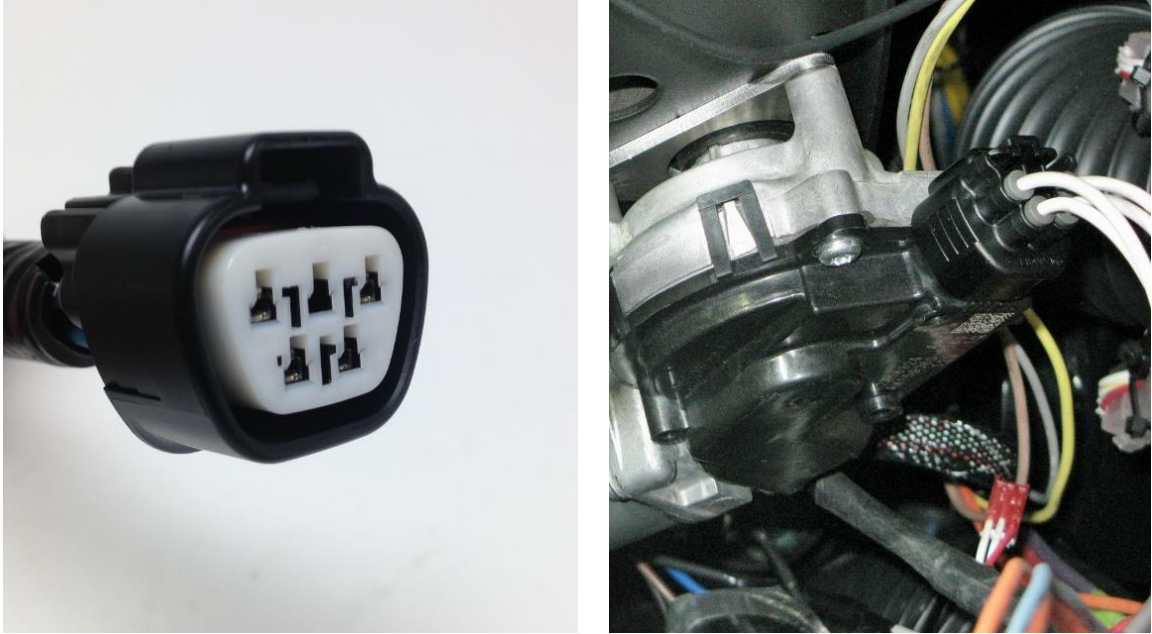
Figure 8 – Wiper Motor Connector
