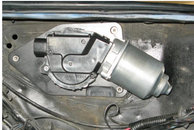
Figure 3 - Wiper Motor Orientation (P/N: 121408 Shown)
