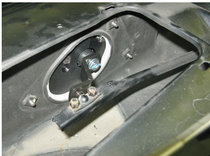
Figure 4 – Attach Pitman Arm to Wiper Linkage
