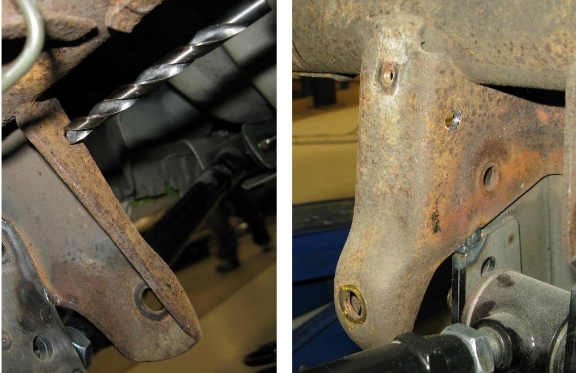
Figure 4 - Drill Factory Axle Bracket
