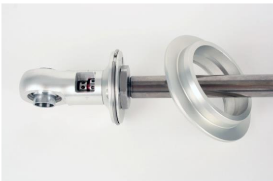
Figure 7 - Remove Upper Spring Seat
