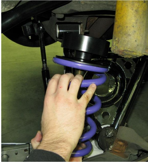
Figure 3 – Install Weight Jack Assembly
