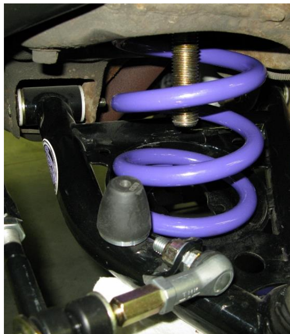
Figure 4 – Weight Jack Assembly Installed
