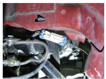
Figure 7 - ABS Body Harness Connector (1993-2002 F-Body)
