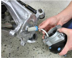
Figure 4 - Position Detroit Speed X-Tracker Hub Assembly (1991-96 Corvette)
