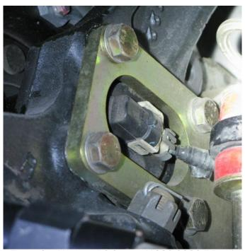
Figure 2 - Unplug ABS Sensor (1993-2002 F-Body)
