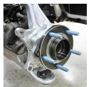
Figure 5 - Install Adapter Assemblies (1991-96 Corvette)
