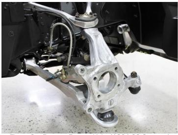
Figure 3 - Remove Factory Hubs (1991-96 Corvette)
