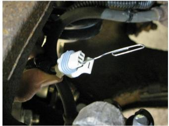
Figure 6 - Remove ABS Terminals (1993-2002 F-Body)
