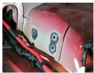
Figure 4 - Drill-Out Spot Welds
