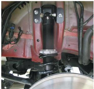
Figure 13 - Install Rear Shocks to Tower Brace
