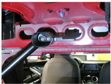
Figure 11 - Attach Upper Mount to Vehicle
