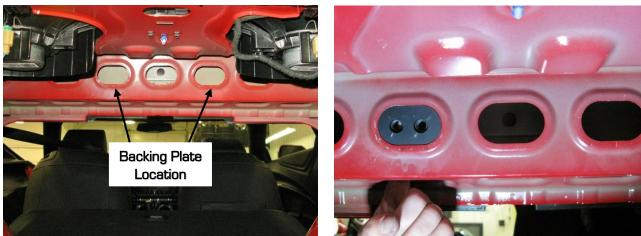
Figure 9 - Position Upper Mount Backing Plate
