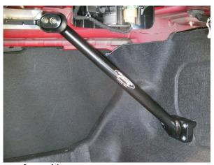
Figure 15 - Tower Brace Assembly
