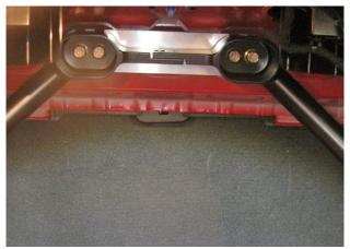
Figure 14 - Install Upper Shim
