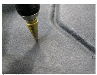
Figure 7 - Drill Spacer Holes
