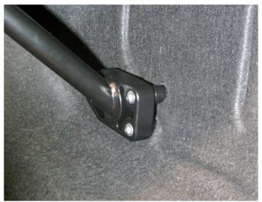
Figure 12 - Install Lower Mount to Vehicle
