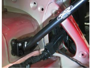
Figure 10 – Position Tower Brace
