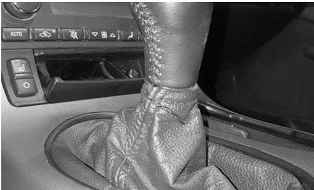
**Then work the boot's elastic cuff** back into the groove on the knob.
