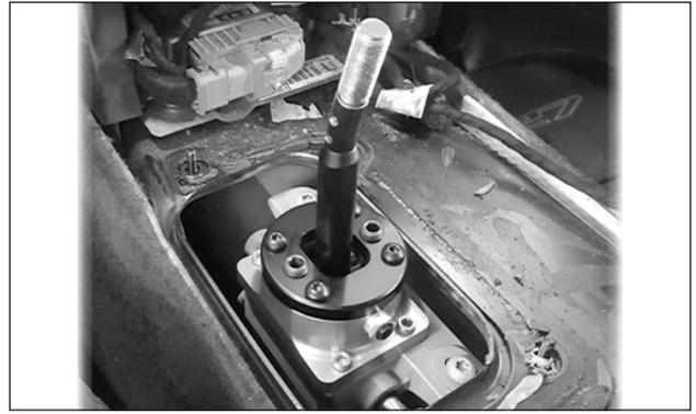
19. Orient the shifter with the lever's bend to the rear, and place it on the shift box, inserting the pivot cup into the shift linkage. Apply medium-strength thread locker to the 4 screws, and use them to secure the shifter to the shift box.
