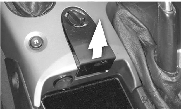
4. **EARLY C6 (2005-2007) ONLY:** At the front edge of the storage compartment, lift up on the rear edge of the half-round panel to detach it from the front console. Disconnect any electrical plugs, and set the panel aside.
