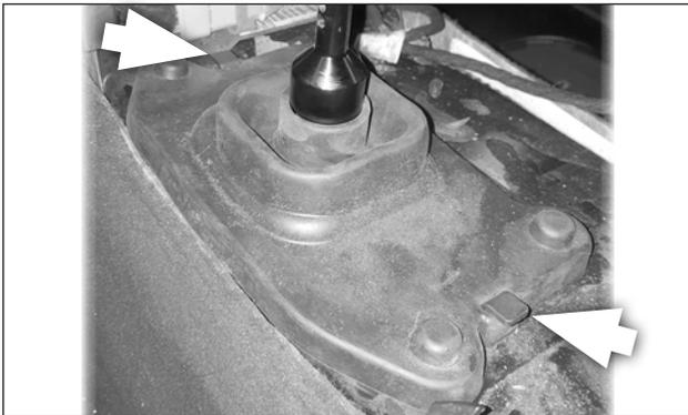
61. Reinstall the sound insulator, pushing its slots down over the tabs on the dust boot.
