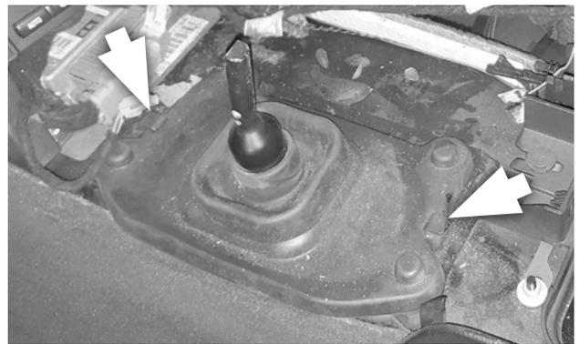
13. Release the sound insulation from its 2 tabs, lift it over the shift lever, and set it aside. (Late C6 molded rubber version shown; early C6 version is flat foam rubber.)
