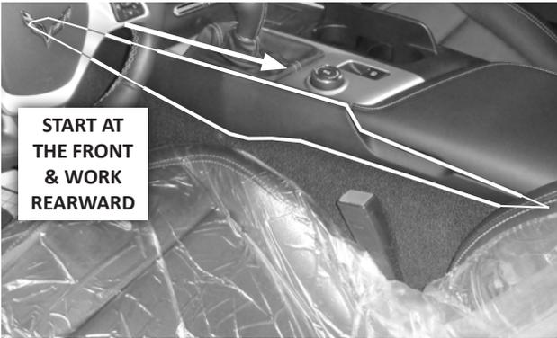
**72. Reinstall the left side trim panel.** First engage the plastic tab at the front. Then, starting at the front of the panel and moving rearward, reattach the 5 friction clips to the console.
