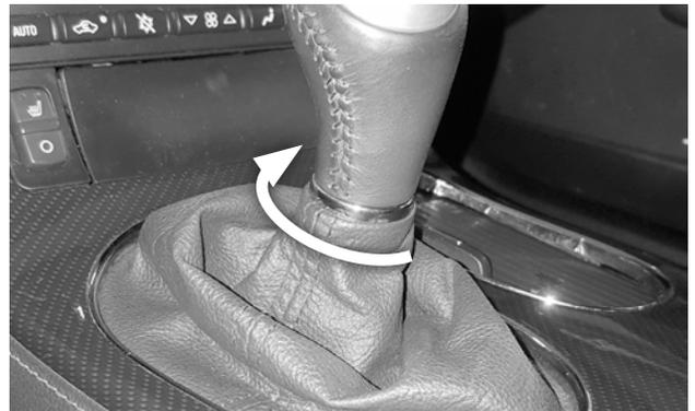
**Then firmly grasp the chrome ring** and turn it 1/4-turn clockwise to lock it into place on the knob.
