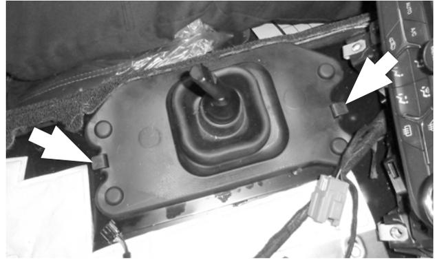
50. Release the sound insulation from its 2 tabs, lift it over the shift lever, and set it aside.
