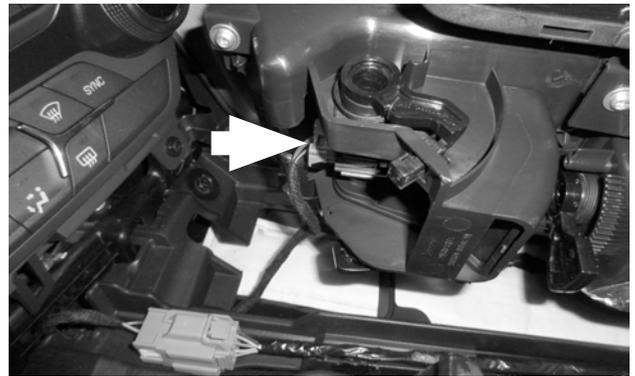
69. Bring the center console panel back into the vehicle and tilt it toward the passenger side. Reconnect the cigarette lighter plug, and check the security of the connection.
