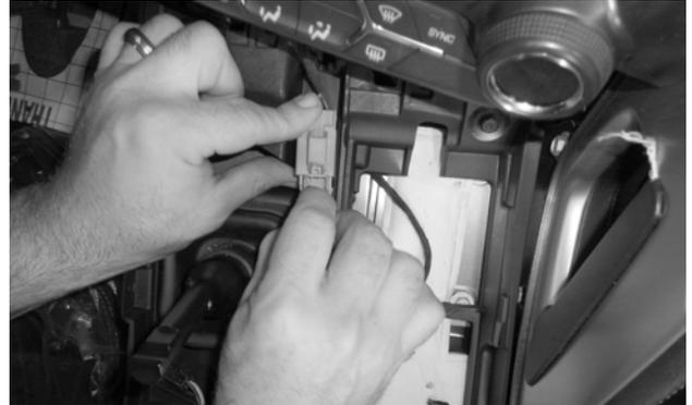
63. Reattach the front harness receptacle to the console base, reconnect the electrical plug, and check the security of the connection
