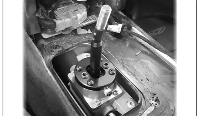
56. Orient the shifter with the lever's bend to the rear, and place it on the shift box, inserting the pivot cup into the shift linkage. Apply medium-strength thread locker to the 4 screws, and use them to secure the shifter to the shift box.
