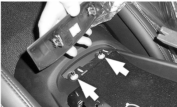
36. **At the rear of the storage compartment**, remove the plastic trim cover, then remove the 2 nuts underneath.
