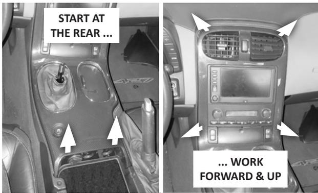
8. Put the shifter in 4th gear and lift the boot opening off the end of the shift lever (to prevent it from catching). Starting at the rear of the front console and working forward, detach it from the console base and dash. Lift up on the rear edges first, then gently pull back on the front edges, just until all the friction clips have been released.
