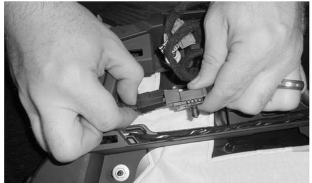
64. Reattach the rear harness receptacle to the console base, reconnect the electrical plug, and check the security of the connection.
