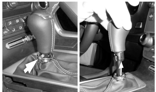
39. **Remove the shift knob screw**, then lift the knob off of the shift lever.
