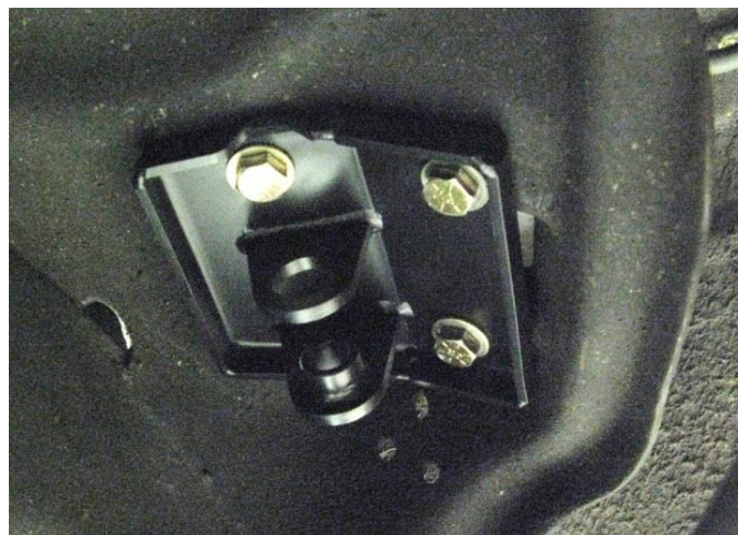
Figure 2 - Installed Upper Coilover Bracket
