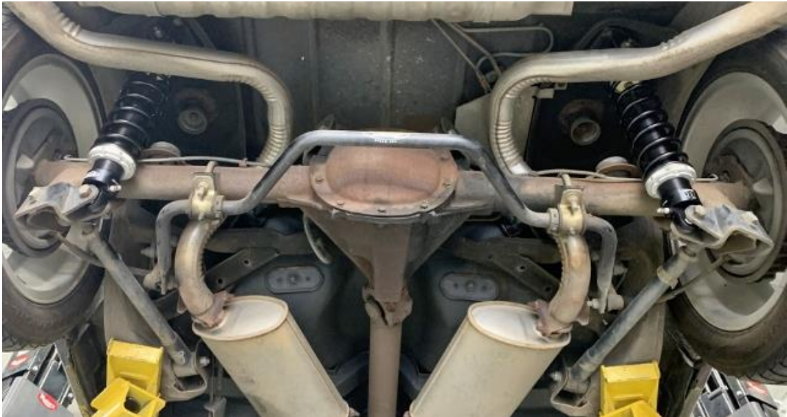
Figure 8 - Completed Coilover Installation
