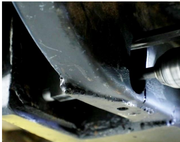
Figure 11 - Drill Bottom Link Hole
