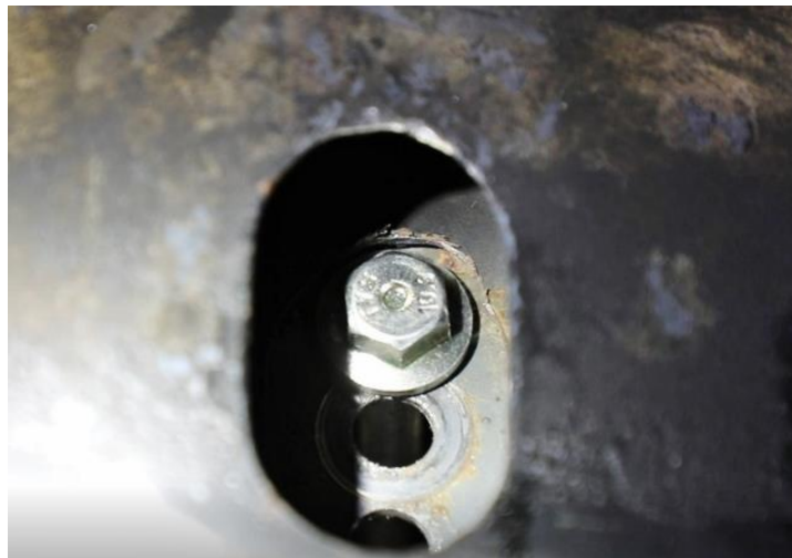
Figure 14 – Grind Bolt Clearance
