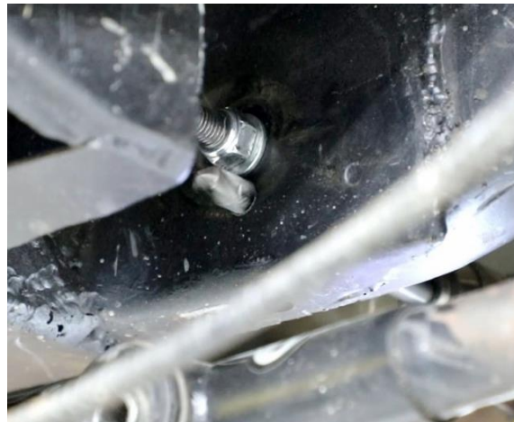
Figure 6 – Drill Bottom Link Hole
