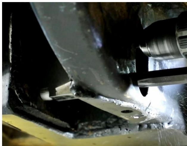
Figure 12 - Drill Top Link Hole
