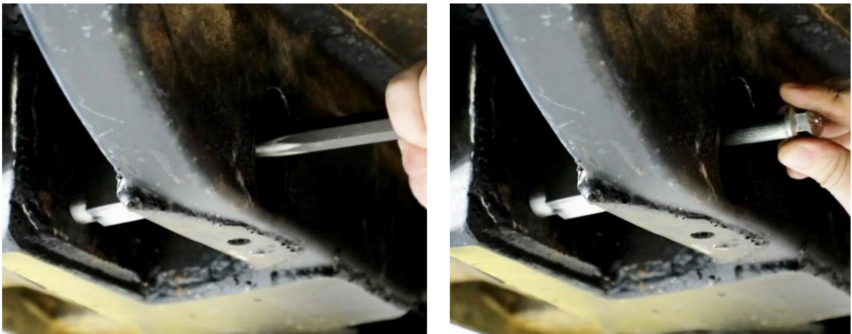
Figure 9 - Install Drill Fixture
