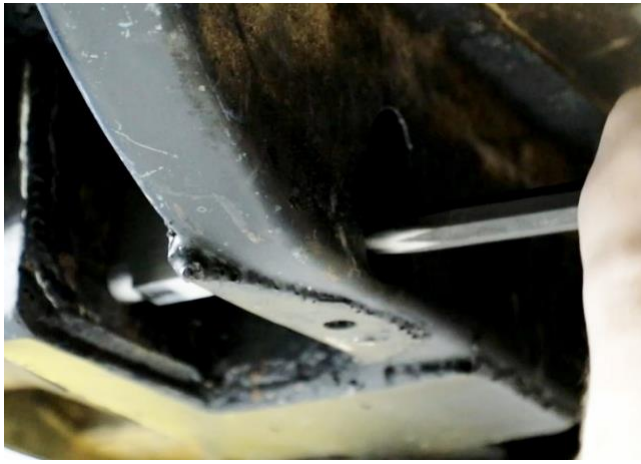
Figure 10 - Align Drill Guide
