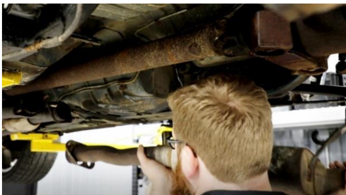
Figure 1 – Remove Exhaust and Parking Brake Clamps
