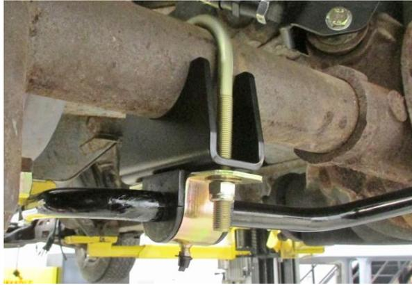
Figure 2 - Install Bar to Bracket
