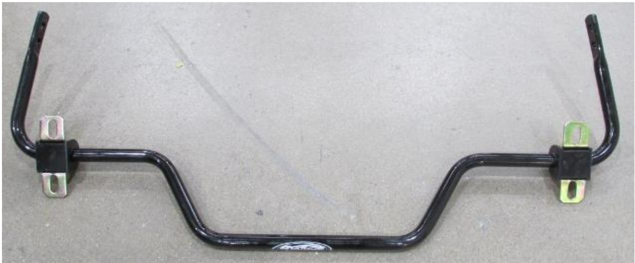
**Figure 1 – Install Bushings and Brackets**
