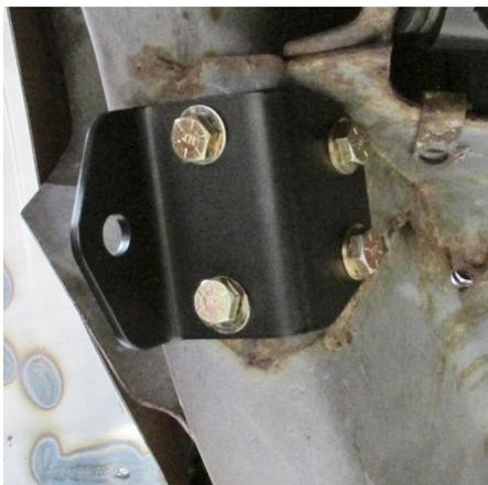
Figure 7 - Install End Link Bracket
