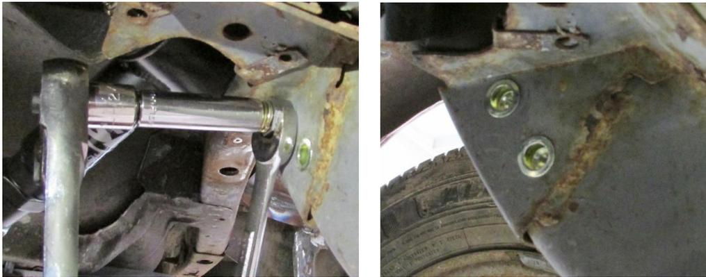
Figure 6 - Install Nut Inserts
