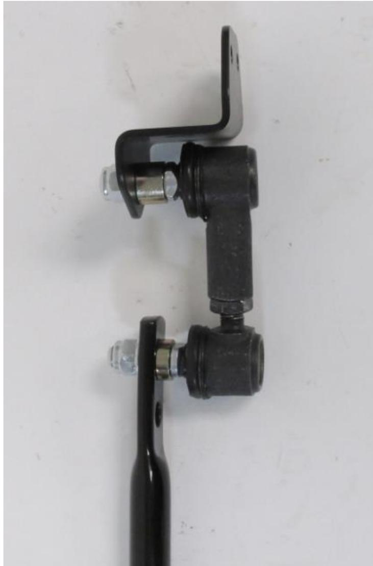
**Figure 8 - Install End Links**
