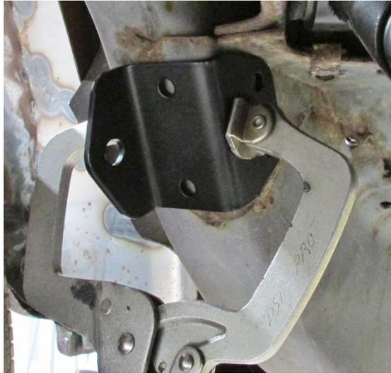
Figure 3 - Locate End Link Bracket
