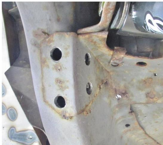
Figure 4 - Drill End Link Bracket Holes
