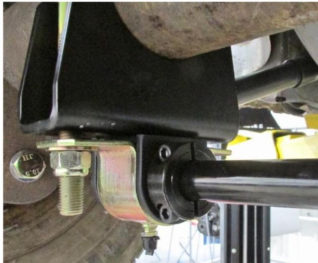
Figure 9 – Install Split Lock Collars
