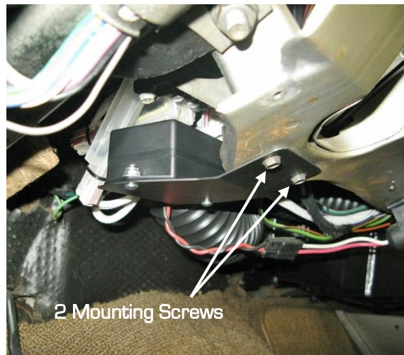
Figure 15 - Install Module & Mounting Plate
