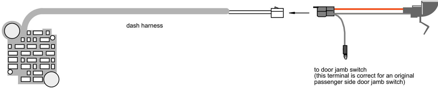
Plug connectors to mating orange/white wires on the dash and rear body wiring, after harnesses have been installed.
