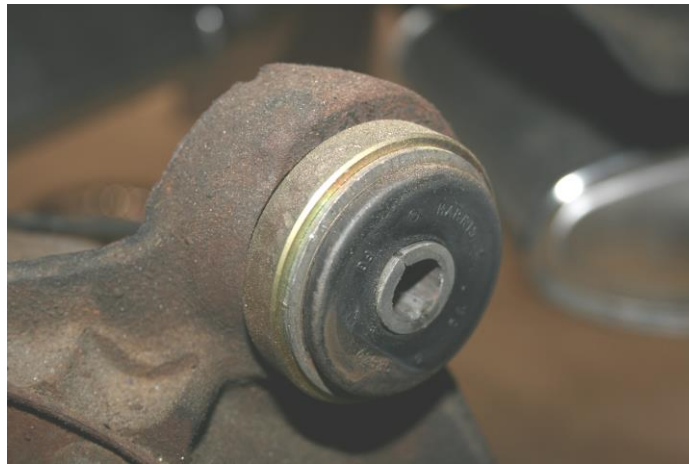
Figure 5 - Replacement Bushing Installed
