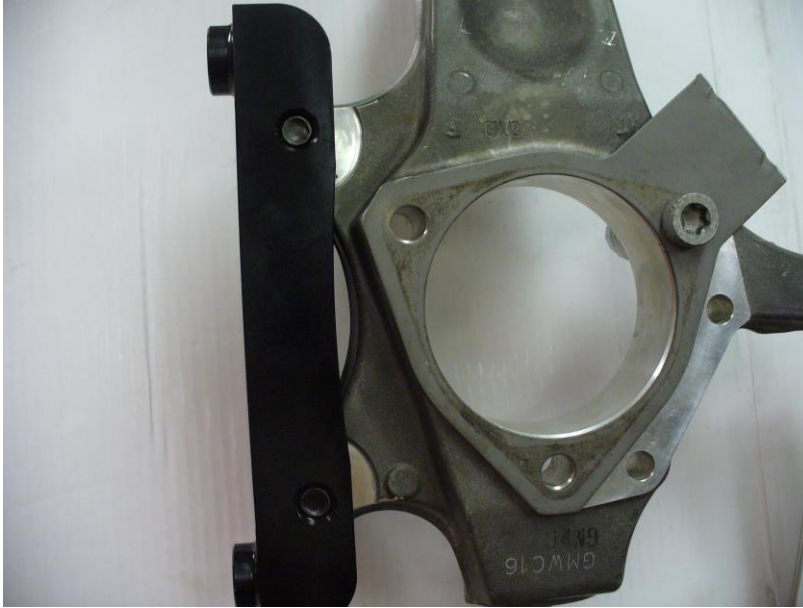
Figure 2: Radial mount bracket installed
