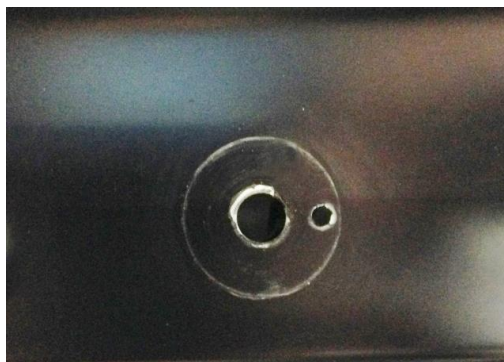
Figure 2 - Drill Anti-Rotation Hole
