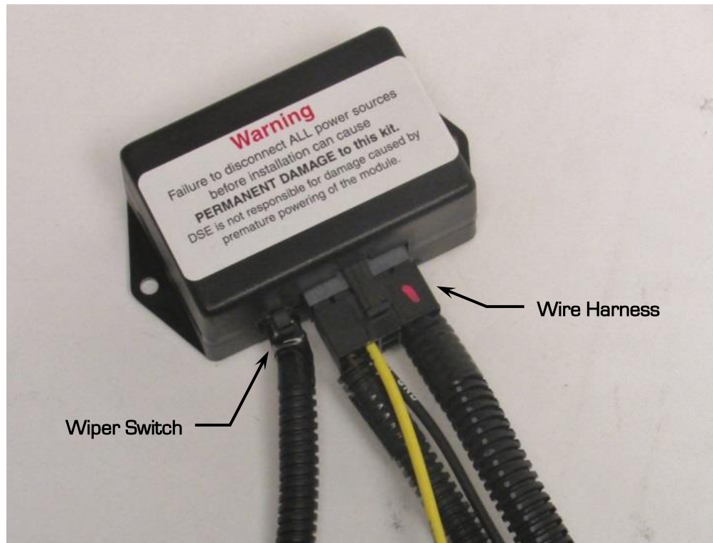
Figure 8 – Connect Wiper Switch & Harness to Module
