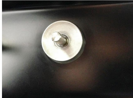
Figure 4 - Thread Bezel onto Switch
