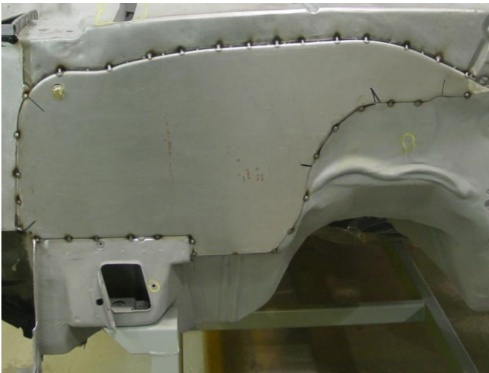
Figure 1 - Panel Tacked in Place
