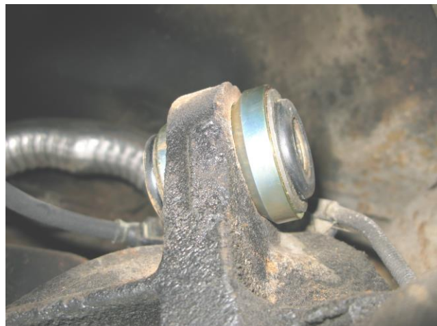
Figure 3 - Replacement Bushing Installed
