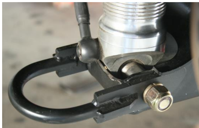
Figure 1 – Installed Tow Hook
