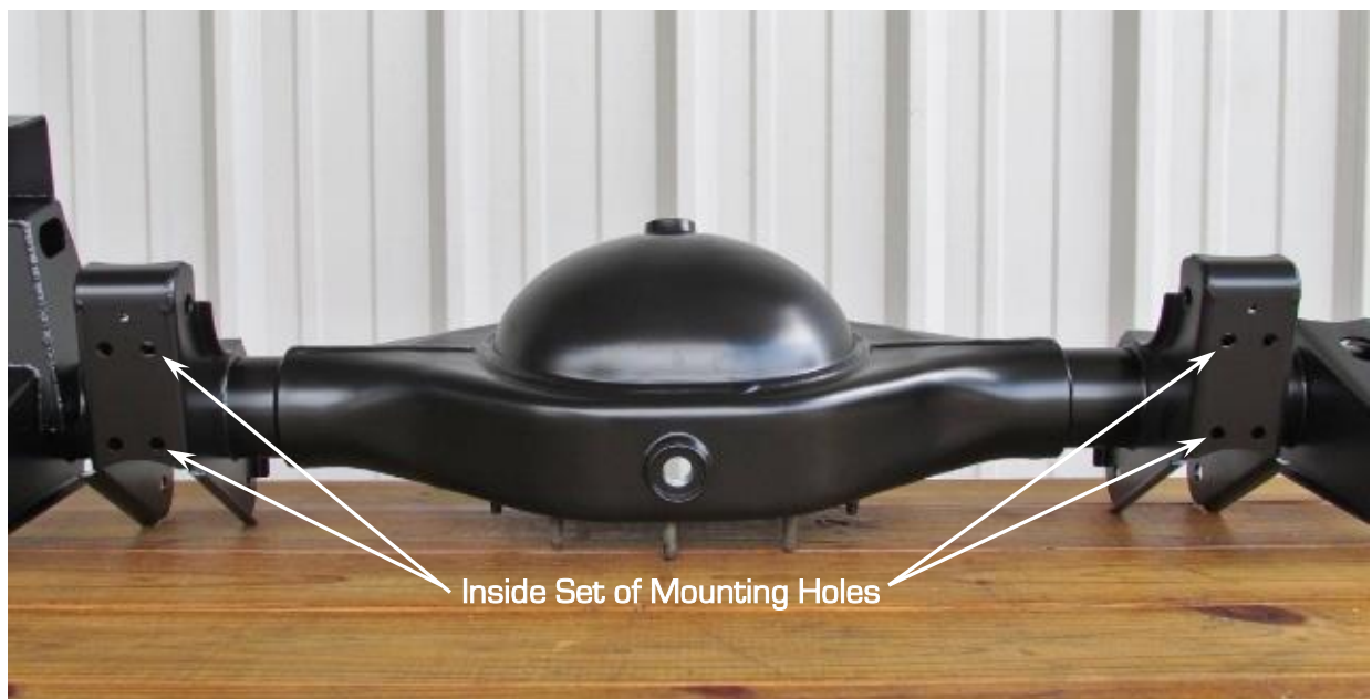
Figure 9 - Use the Inside Set of Holes to Mount the Sway Bar Bracket
