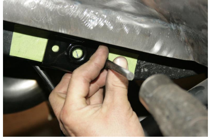
Figures 5a and 5b – Locating the Sway Bar Mounting Bracket Holes on the Frame Rail
