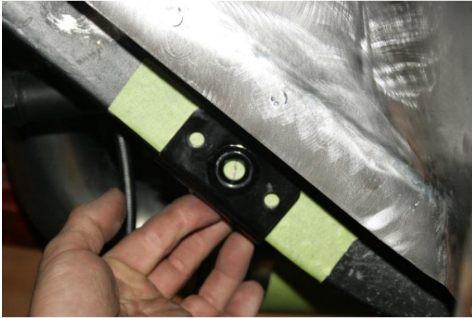
Figures 5a and 5b – Locating the Sway Bar Mounting Bracket Holes on the Frame Rail
