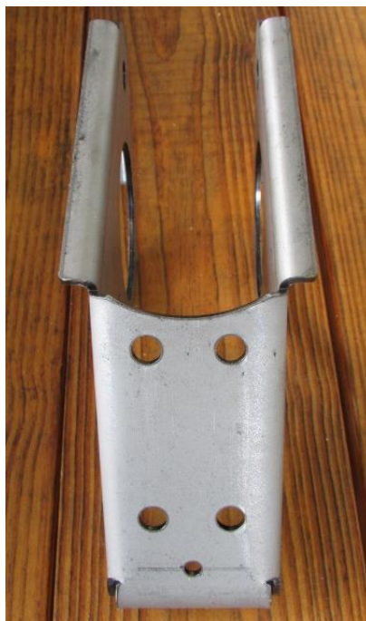
Figure 1 - Pre-Drilled Holes in Coilover Bracket
