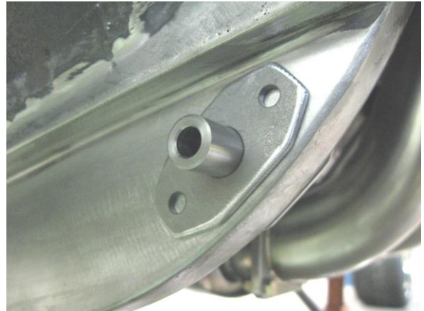
Figure 5 – Locating the Frame Insert on the Outside Frame Rail
