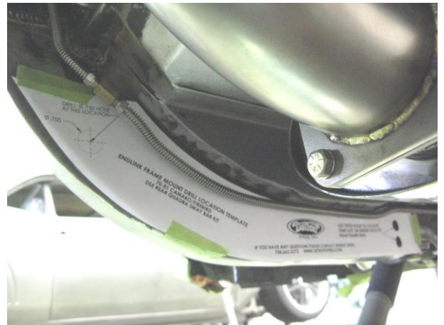
Figure 2 – Positioning the Template on the Frame Rail
