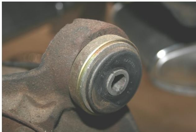
Figure 5 - Replacement Bushing Installed
