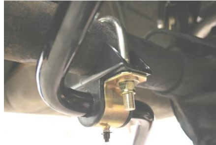
Figure 4 – Sway Bar Mounted on Rear Axle
