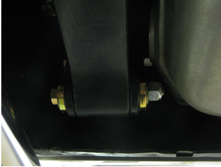
Figure 2 - Rear Leaf Spring Shackles Installed
