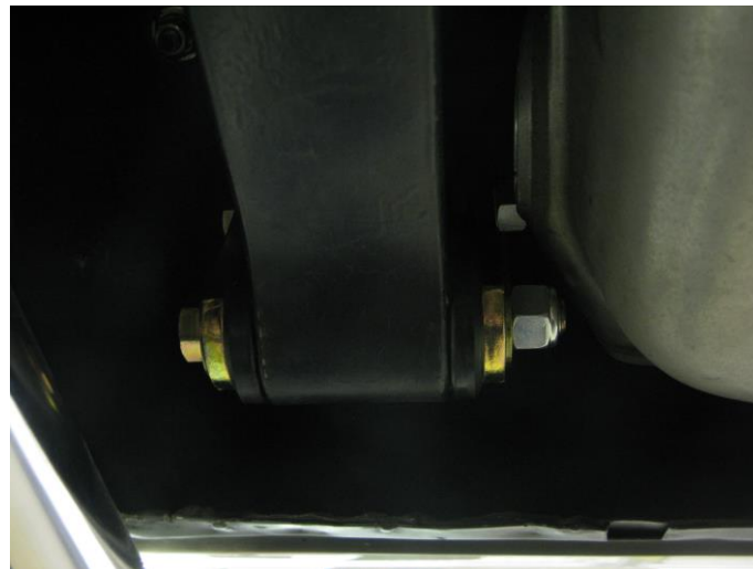
Figure 2 - Rear Leaf Spring Shackles Installed
