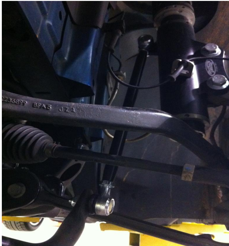
Figure 2 - Picture above shows the LH endlink installed
