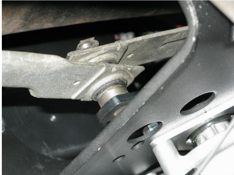
Figure 6 - Attach Wiper Linkage to Pitman Arm
