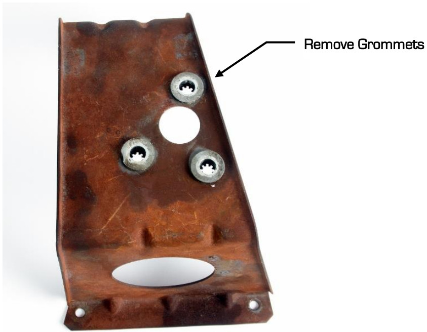
Figure 2 - Factory Wiper Motor Mounting Bracket
