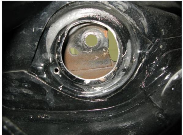
Figure 5 - Modified Shock Pass Through
