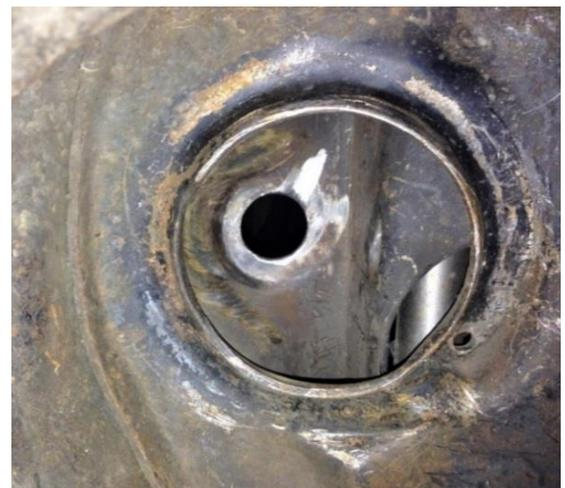
Figure 6 - Remove Sharp Edges/Burrs
