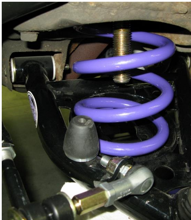
Figure 4 – Weight Jack Assembly Installed
