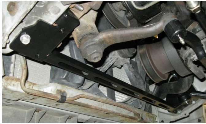
Figure 2 - Front Frame Bracket
