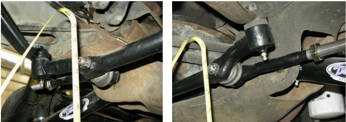
Figure 3 - Level the Center Link
