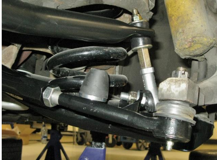
Figure 5 – Sway Bar End Link with DSE Lower Control Arm
