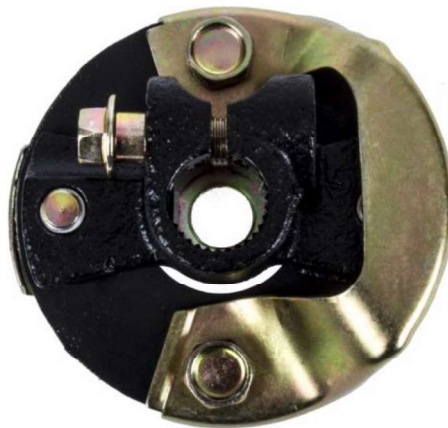
Figure 1 - DSE Rag Joint
