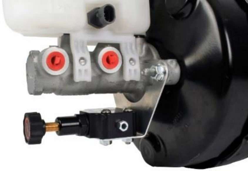
Figure 1 - Completed Bracket Installation
