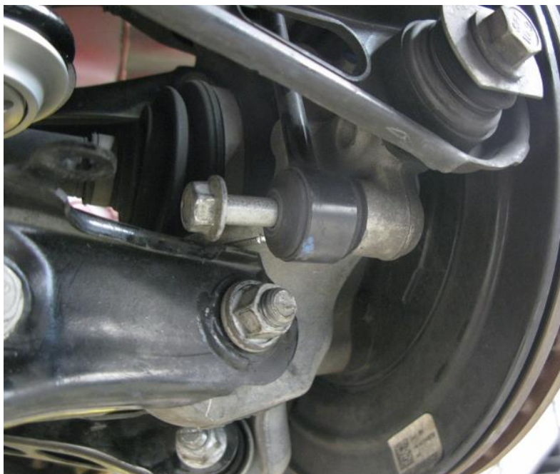
Figure 18 - Re-attach Sway Bar End Links
