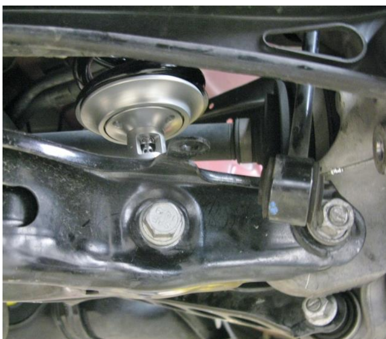
Figure 17 - Re-attach Lower Control Arm & Trailing Link
