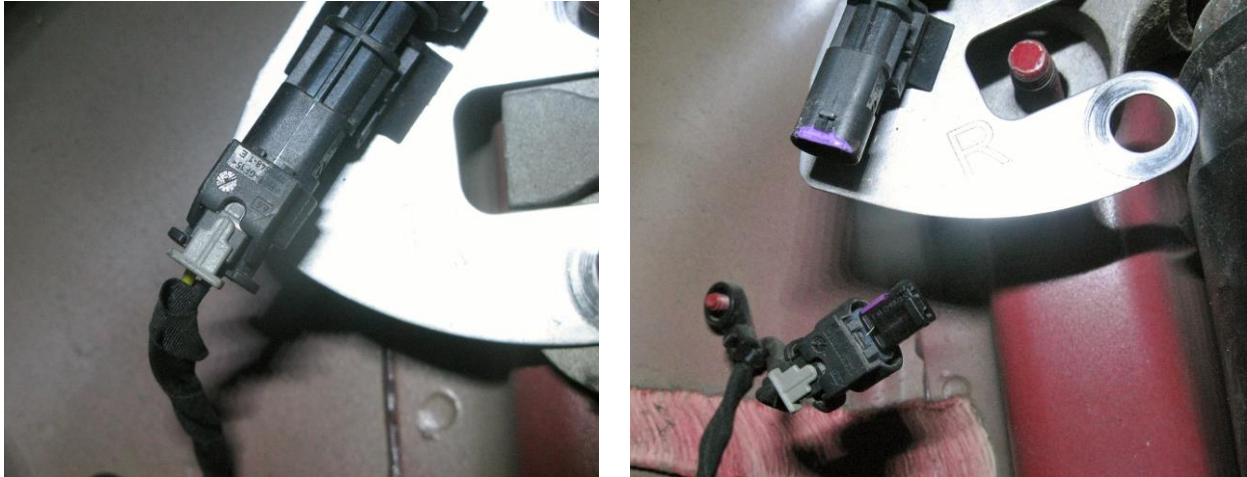
Figure 7 – Disconnect Magnetic Ride Control
