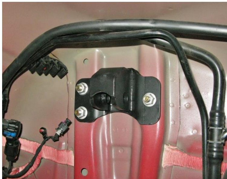
Figure 10 - Install Upper Shock Mount
