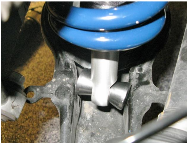
Figure 16 - Install Tapered Spacers
