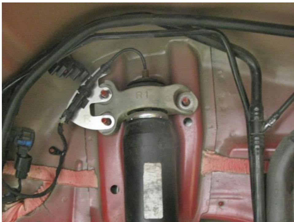
Figure 6 - Remove Upper Shock Mount Nuts
