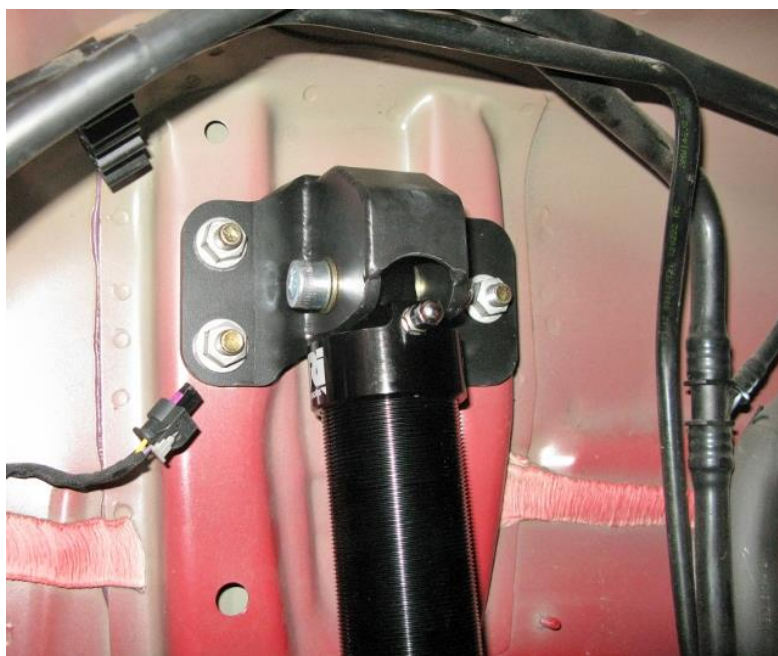
Figure 15 - Install Coilover Shock
