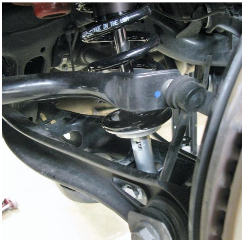
Figure 19 - Final Coilover Shock Assembly
