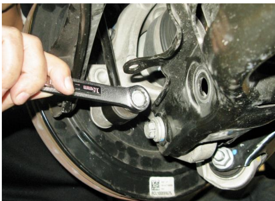
Figure 4 - Disconnect Sway Bar End Links
