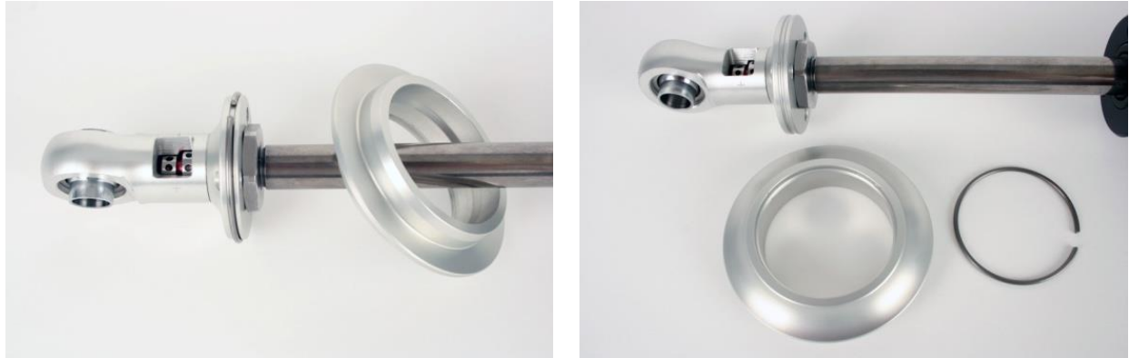
Figure 11 – Remove Spring Seat & Retaining Ring
