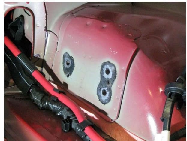
Figure 4 - Drill-Out Spot Welds
