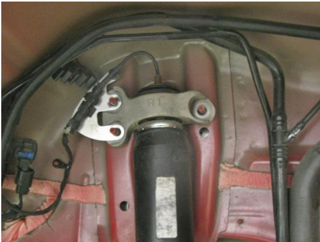
Figure 6 - Remove Upper Shock Mount Nuts
