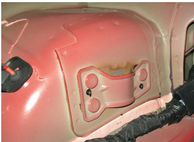
Figure 4 - Drill-Out Spot Welds
