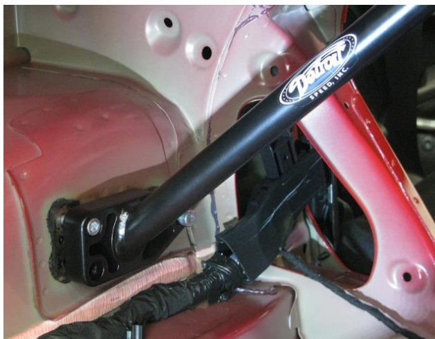
Figure 10 – Position Tower Brace
