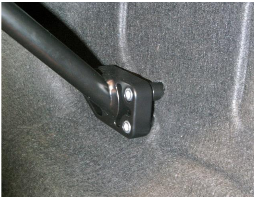
Figure 12 - Install Lower Mount to Vehicle
