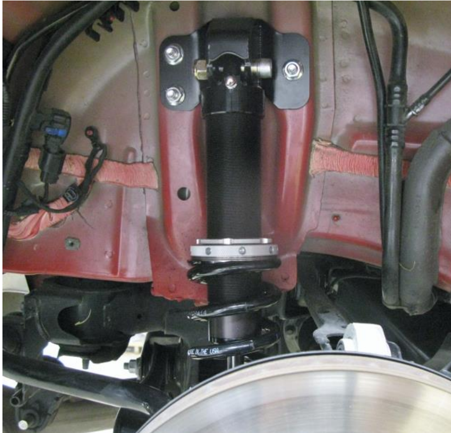
Figure 13 – Install Rear Shocks to Tower Brace
