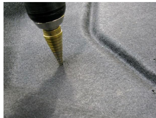
Figure 7 - Drill Spacer Holes
