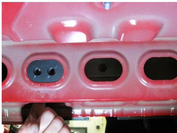
Figure 9 – Position Upper Mount Backing Plate
