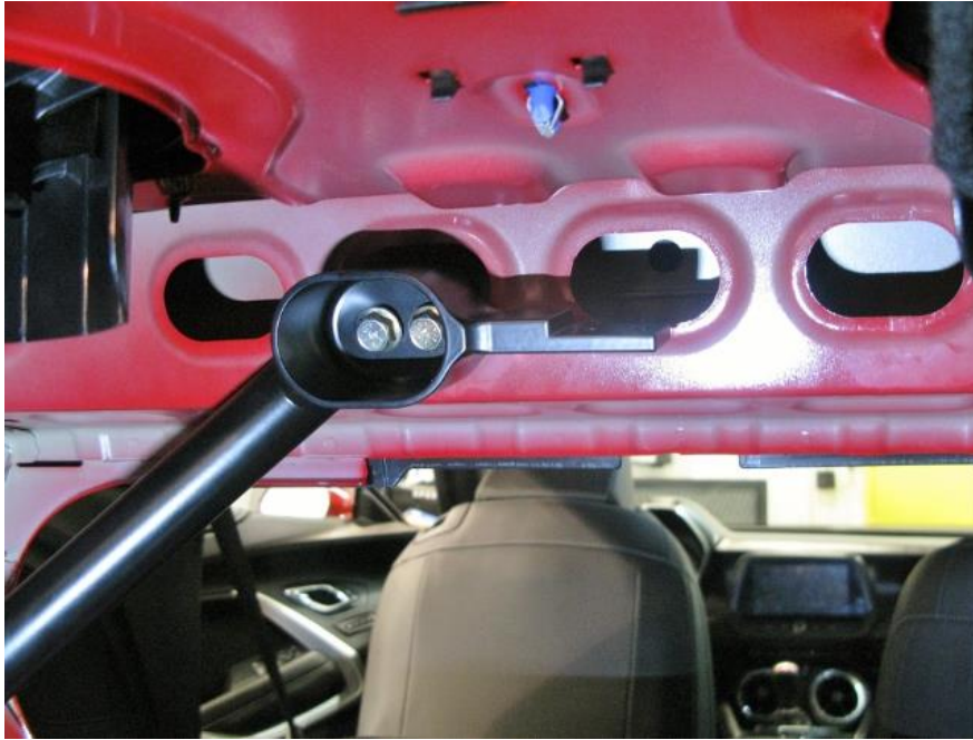
Figure 11 - Attach Upper Mount to Vehicle
