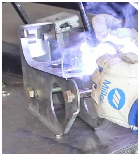
Figure 2 – Weld Axle Bracket Reinforcement
