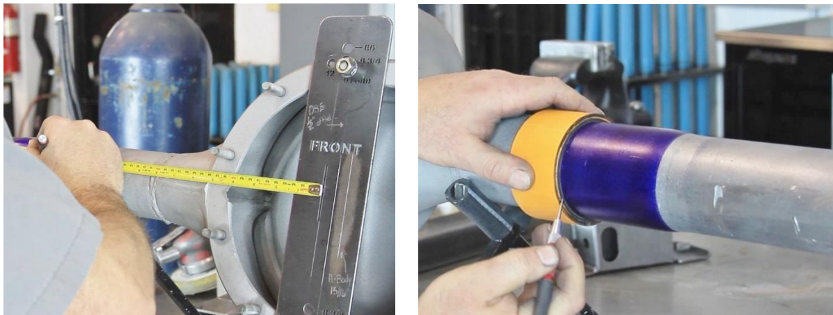
Figure 3 - Locate Axle Brackets on Axle Tubes
