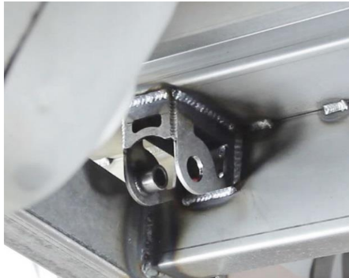
Figure 6 - Weld Upper Shock Mounts
