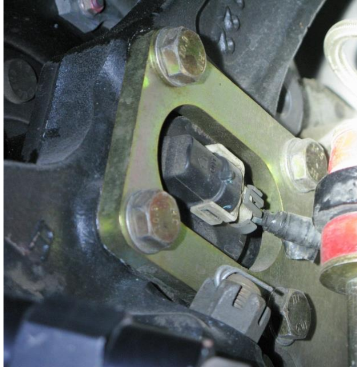
Figure 2 – Unplug ABS Sensor (1993-2002 F-Body)
