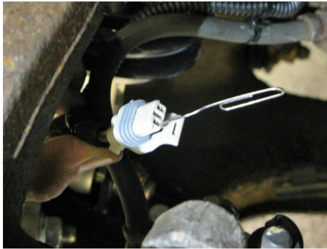
Figure 6 - Remove ABS Terminals (1993-2002 F-Body)
