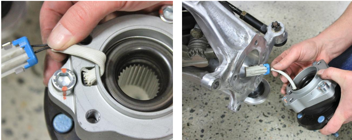
Figure 4 – Position Detroit Speed X-Tracker Hub Assembly (1991-96 Corvette)
