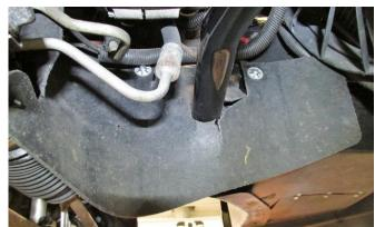
Figure 8 - Re-Install Splash Shield
