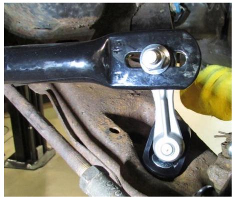
Figure 5 - Attach End Link to Sway Bar
