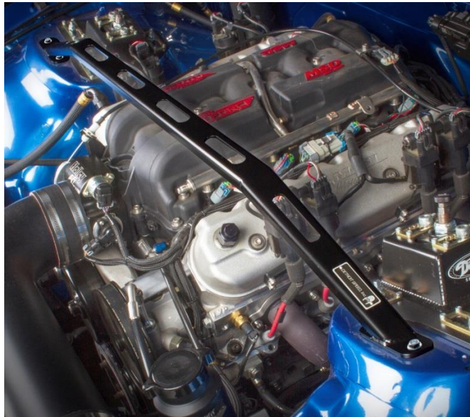
Figure 5 - Install Strut Tower Brace
