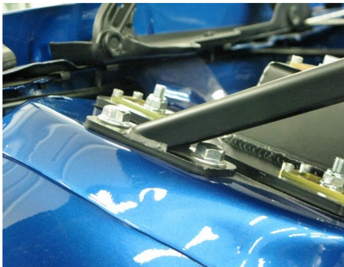
Figure 3 - Install M10 Fasteners
