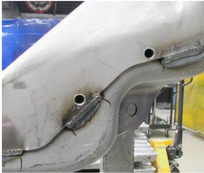
Figure 3 - Drill Frame Stand Holes
