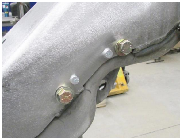
Figure 7 – Test Fit Drilled Holes
