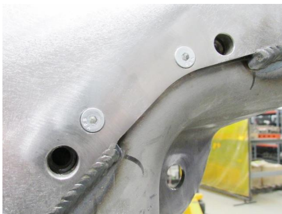
Figure 8 – Countersink Nut Plate Holes
