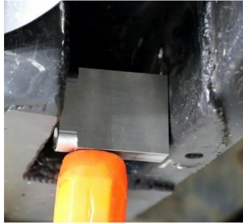
Figure 8 - Place Fixture in Link Pocket
