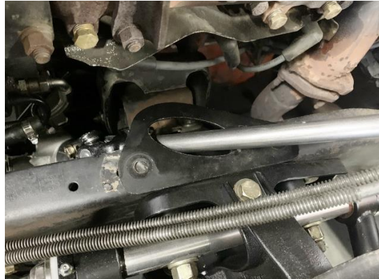
Figure 2 – Position Splined Shaft
