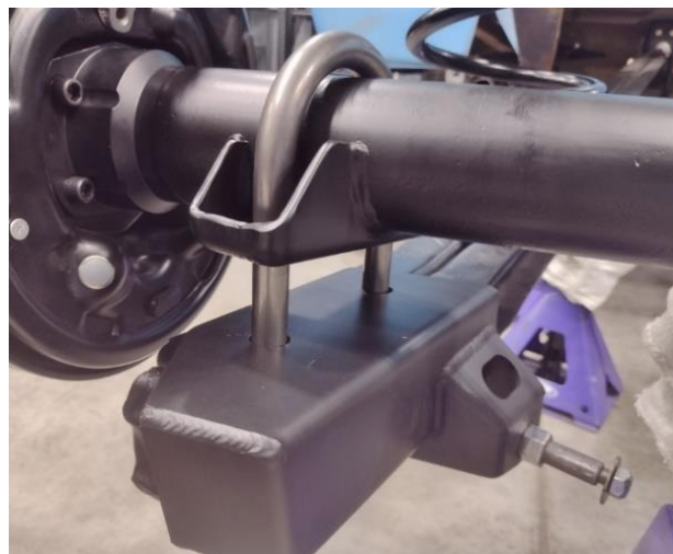
Figure 9 - Raise Trailing Arm
