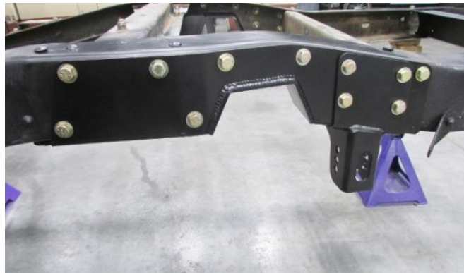
Figure 12 - Install Track Bar Bracket
