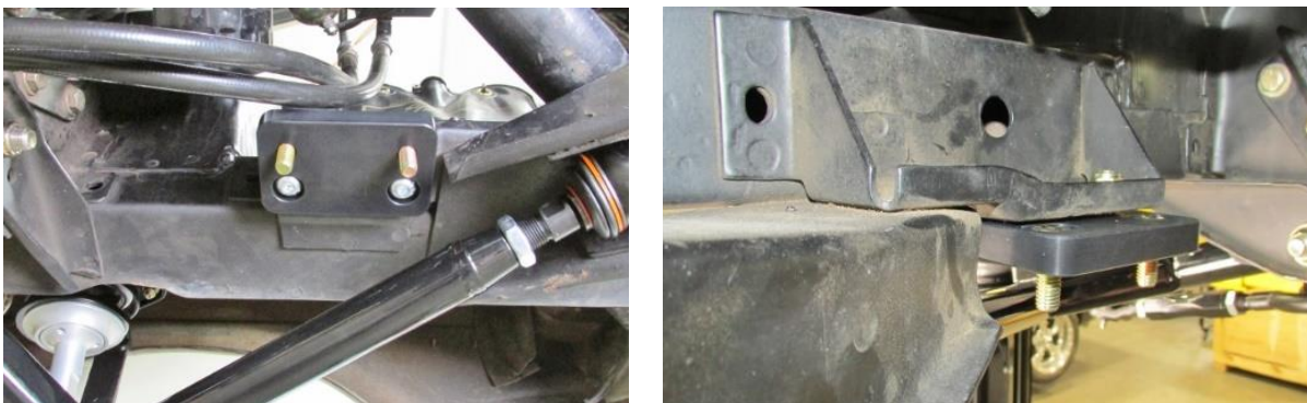
Figure 2 –Sway Bar Mount Spacer Installed
