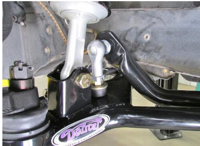
Figure 7 – Install End Link to Sway Bar
