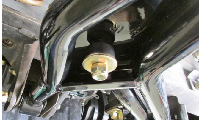
Figure 6 – Install End Link Hardware
