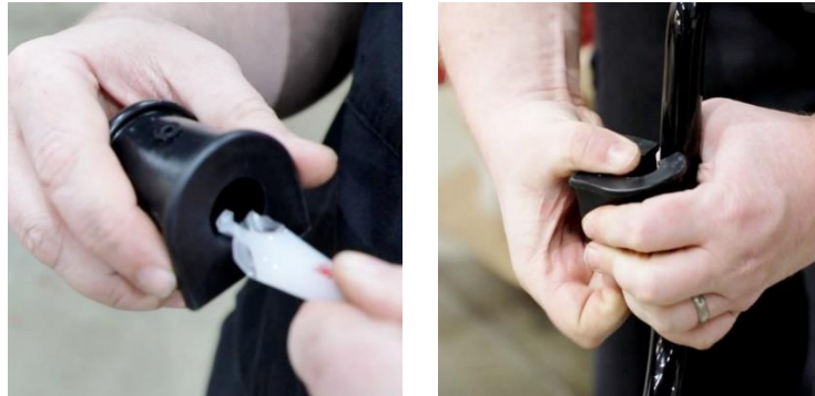
Figure 3 - Grease & Install Bushings
