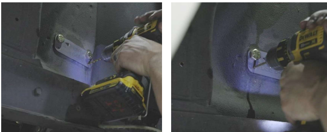
Figure 4 – Mark Drill Locations
