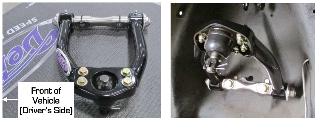
Figure 13 - Install Upper Control Arms
