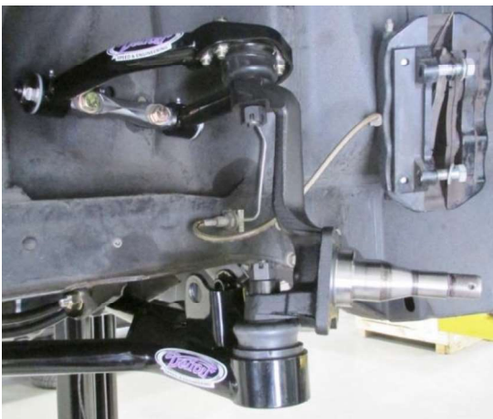
Figure 23 – Torque Castle Nuts
