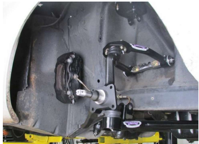
Figure 23 – Torque Castle Nuts
