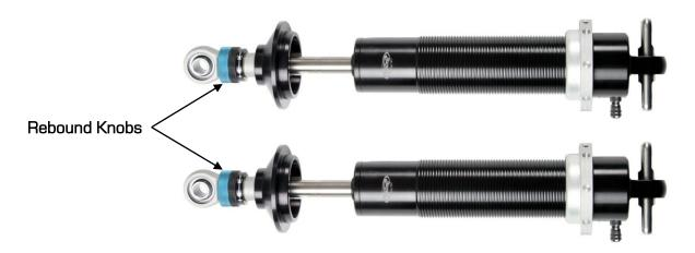
Figure 11a- Detroit Speed Single Adjustable Shock
