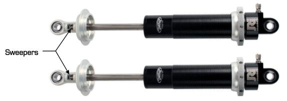
Figure 12a – Detroit Speed Double Adjustable Shock
