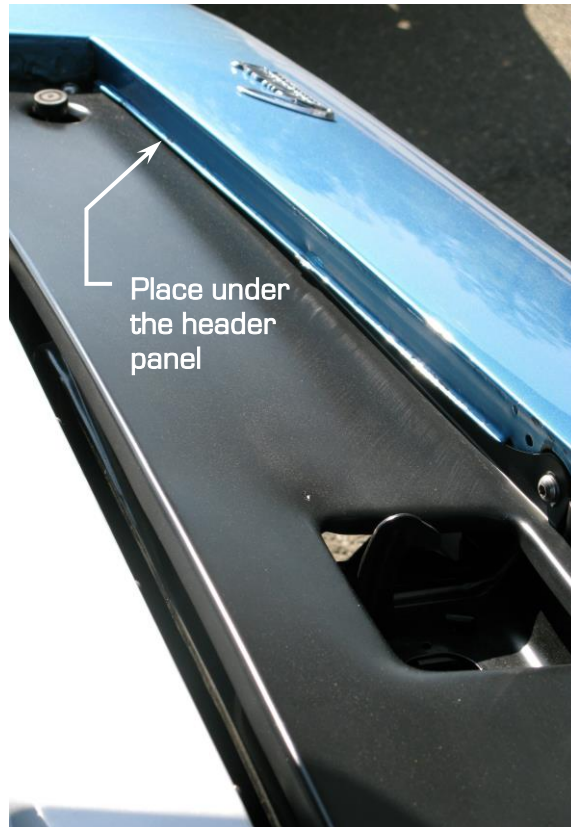
Figure 1 – Core Support Closeout under the Header Panel
