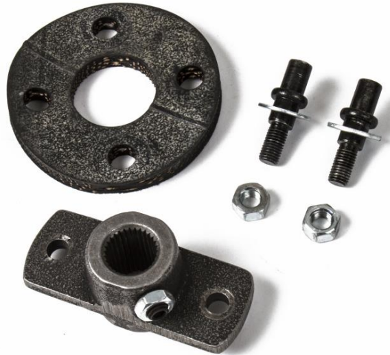
Figure 2 - Separate the Rag Joint from the Coupler
