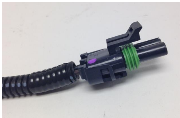
Figure 8 – Washer Pump Connection
