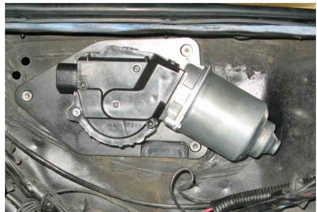
Figure 3 - Wiper Motor Orientation (P/N: 121408 Shown)
