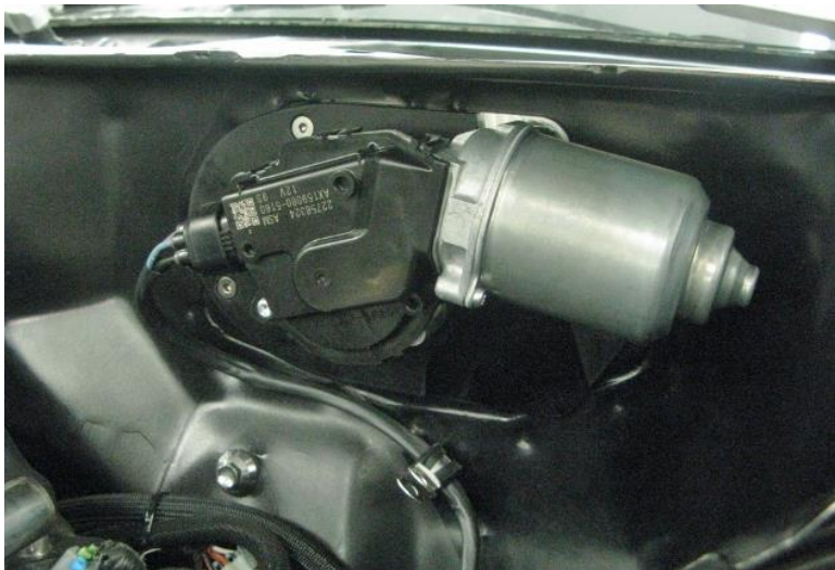
Figure 7 – Install Wiper Motor Connector (P/N: 121406 Shown)
