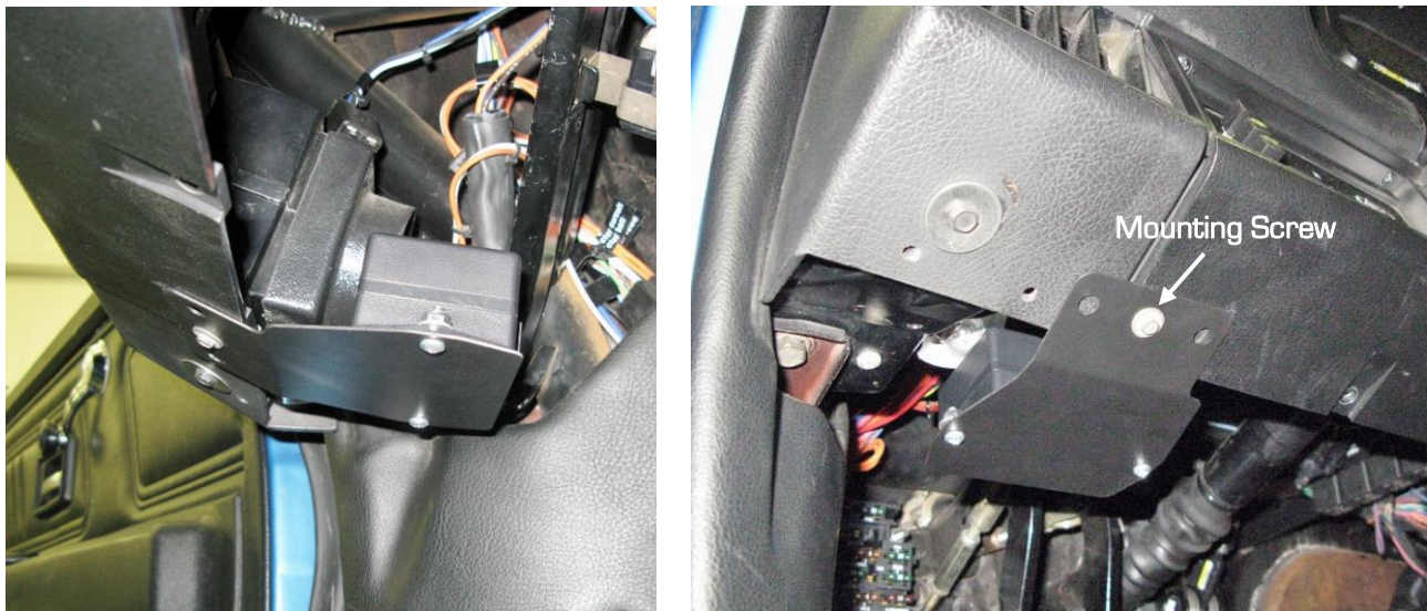
Figure 10 - Install Module & Mounting Plate
