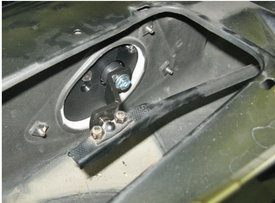
Figure 4 – Attach Pitman Arm to Wiper Linkage
