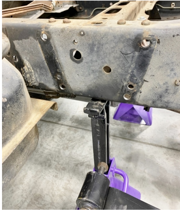
Figure 2 - Drill Out Frame Holes
