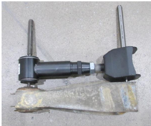
Figure 5 – Detroit Speed vs. Stock Upper Link
